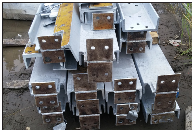
Masked faying surfaces used in high strength structural connections.
