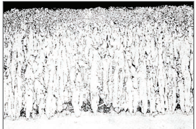
Figure 2: Atypical zinc-iron alloy layers
