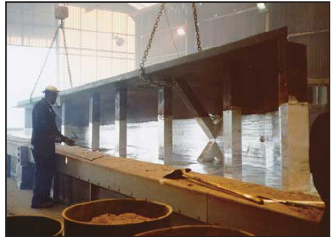
Progressive dipping increases the maximum size that can be HDG
