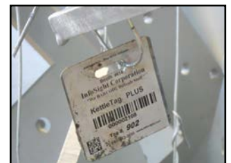
Figure 40: Metal barcode tags designed to withstand the HDG process can be easily removed.
